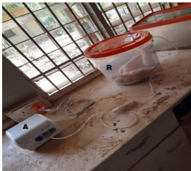
Plate I: Inhalation chamber; A: Human nebulizer and B: Improvised inhalation bucket containing the rats
